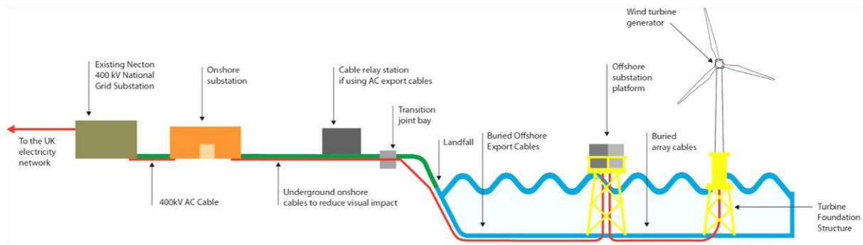
Figure 1 Diagram illustrating the key components of the Norfolk Boreas project
