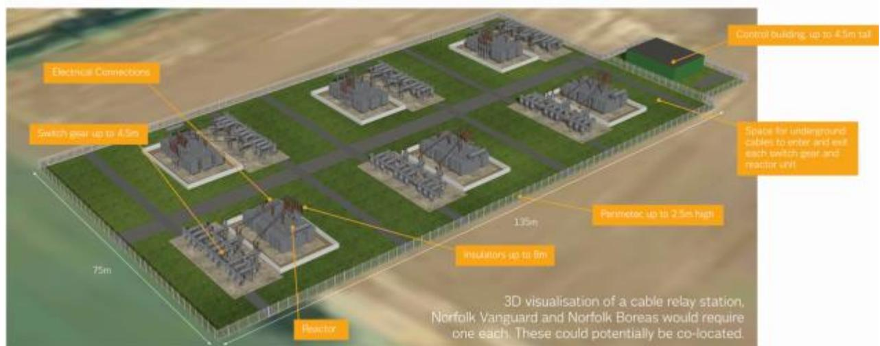
**Figure 4 visualisation of cable relay station**
