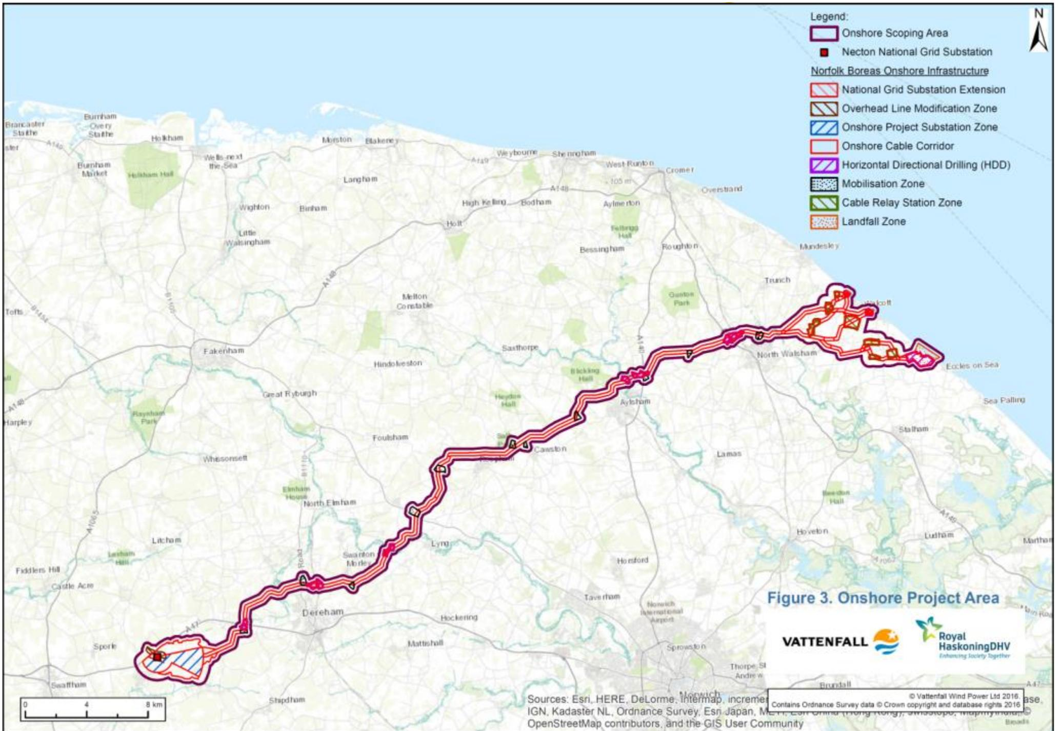
Up to six offshore export cables operating at between 220 and 245 kilovolts will be used to transmit the electricity to shore. Export cables would make landfall at one of the three locations currently being considered. These are:
